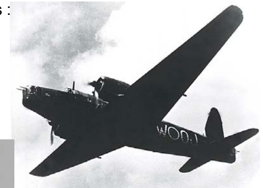
Vickers Wellington P = 2 x 1055CV Vmax = 410km/h Plafond = 6700m Charge utile = 2040kg
