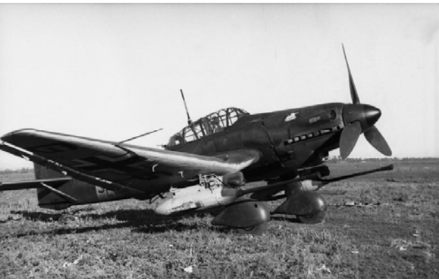
Junkers 87 Stuka P = 1200CV Vmax = 310km/h Plafond = 8000m Charge utile = 500kg
