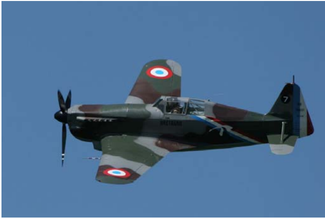
Morane Saulnier MS406 P = 860CV Vmax = 486km/h Plafond = 9850m Charge utile = 700kg
