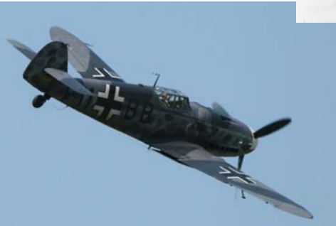
Messerschmitt Bf109 P = 1175CV Vmax = 560km/h Plafond = 10500m Charge utile = 600kg
