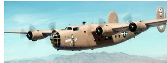
Consolidated B24 Liberator 1941 4 x 1200CV – 470km/h - 8500m 2300kg de bombes
