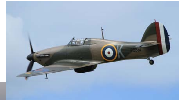
Hawker Hurricane P = 1300CV Vmax = 510km/h Plafond = 11000m Charge utile = 800kg
