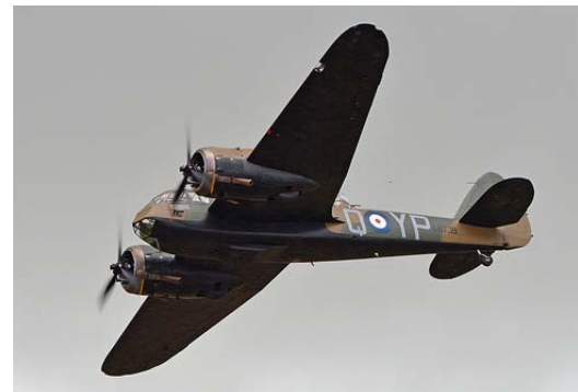
Bristol Blenheim P = 2 x 840CV Vmax = 450km/h Plafond = 8500m Charge utile = 450kg
