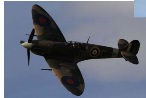
Supermarine spitfire P = 1040CV Vmax = 557km/h Plafond = 9300m Charge utile = 600kg
