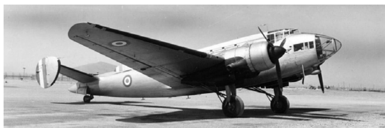
Lioré et Olivier LeO 45 P = 2 x 1060CV Vmax = 495km/h Plafond = 9000m Charge utile = 3600kg
