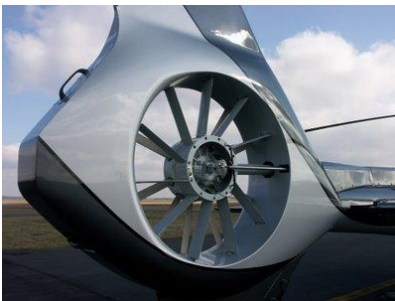
Rotor anti-couple "fenestron"
